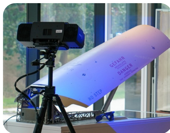
Figure 15. Setup of the VAS System projecting onto an Eurofighter Airbrake.
