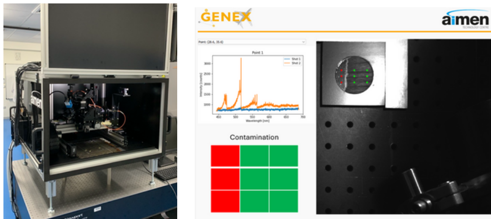
Figure 17. (Left) Stand-alone and out-of-the-lab LIBS system implementation; (Right) Software interface for control and LIBS analysis
