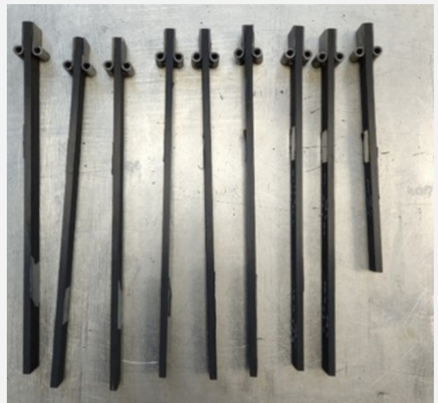
DCB specimens manufactured for the test
