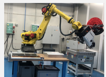
Automated Tape Laying (ATL) of 3R tapes for in-situ consolidation
