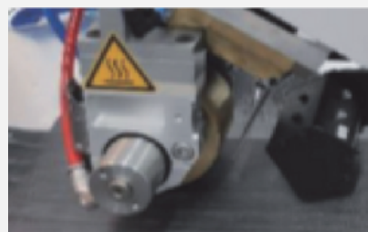
Automated Tape Laying (ATL) of 3R tapes for in-situ consolidation
