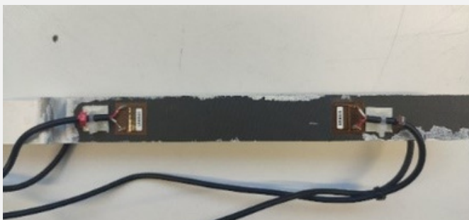
DCB specimen instrumented with MFC transducers to perform UGW tests that will be used to validate FE simulations
