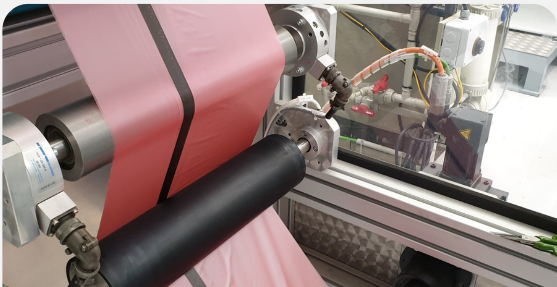
Recyclable 3R composite tapes with embedded Fiber Optic Sensors (FOS)
